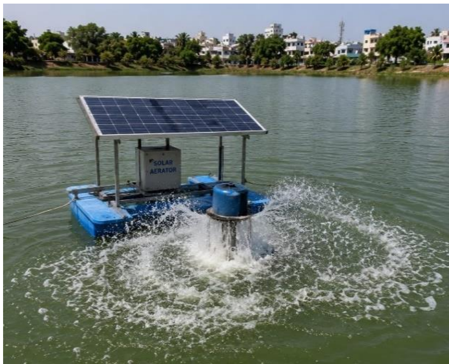
Figure 5: Solar Aerator for cleaning of lake
