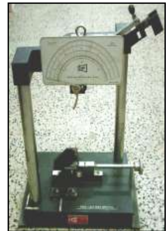
Figure-4: Impact Test Instrument
