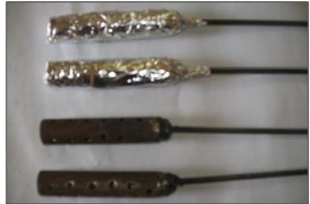
Figure 2: Photograph of perforated mild steel capsule welded to plunger rod (below), Mg or SiC particles inside the capsule shown wrapped with Al foil (top)
