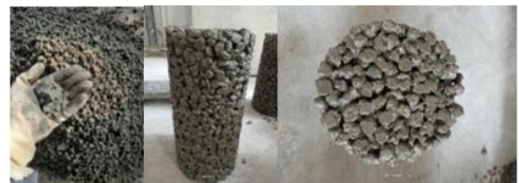
Figure 1: A model of the homogeneity for the mixtures and pervious concrete samples floor
