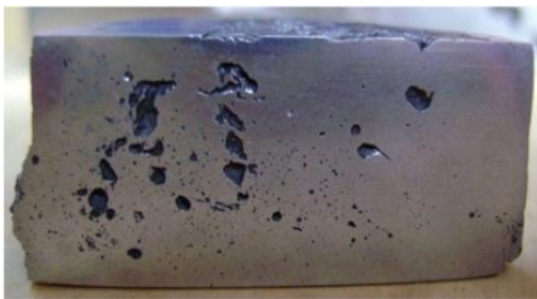
Figure 1: Porosity defects in aluminum casting results
