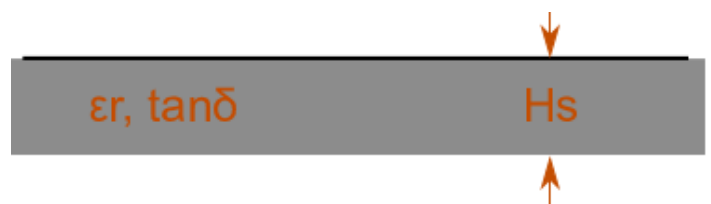
Figure 2(c): View of meander-line antenna from the side
