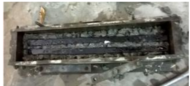
Figure 6: Bamboo coated with coal tar placed in beam
