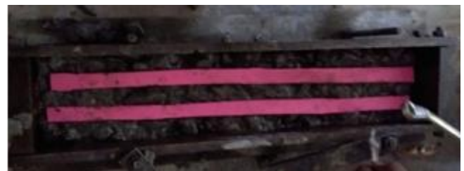
Figure 7: Bamboo coated with resin placed in the beam
