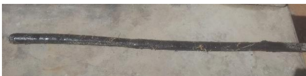
Figure 4: Bamboo coated with coal tar
