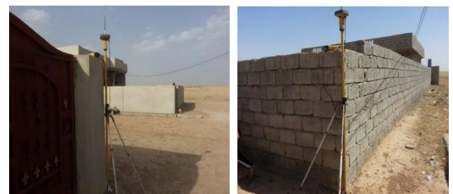
Figure 3: Using a D.G.P.S Device to Determine a Set of Points in the Mosul District, Ulmash Subdistrict
