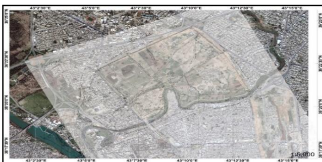
Figure 17: Image of a Cadastral Map Spatially Corrected According to the GCS_WGS_1984 System [2]
