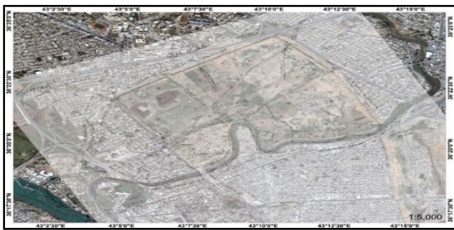
Figure 16: Image of a Cadastral Map Spatially Corrected According to the GCS_Clarke_1880 System [2]
