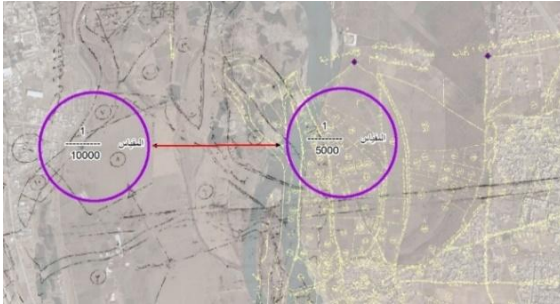
Figure 11: The difference between the boundaries of the Yarmja Northern District, scale 1:5000, and the Harakia and Forests, scale 1:10000 [2]
