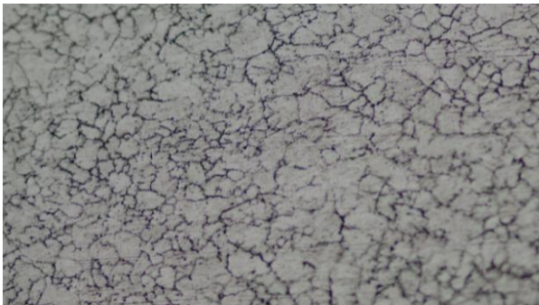
Figure 8: Results of metallographic testing near the failure coil spring 500X magnification scale
