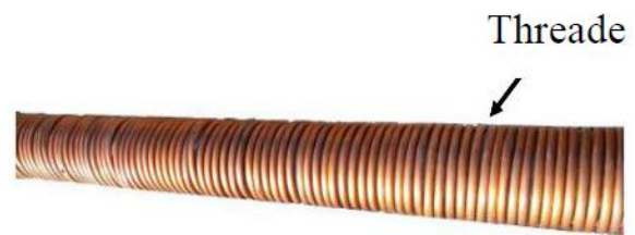
Figure 4: The threaded copper tube used in the pickup
