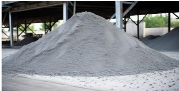
Figure 3: Fly Ash used for stabilization
